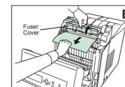
If the paper has jammed inside the duplex unit, as shown in C, lift the duplex unit and remove the paper by holding it in the middle.
