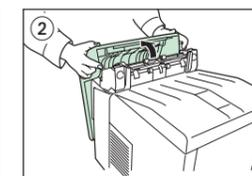
If the paper has jammed inside the fuser unit, as shown in B, open the fuser cover and remove the paper by pulling its edge.
